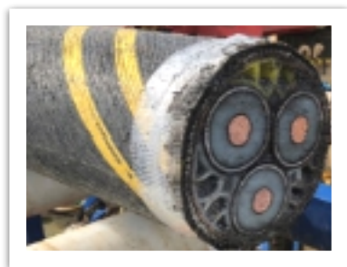
• Figure 6. Cross section of subject cable
