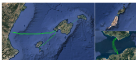
Fig. 1. Location of the submarine power cables in the Spanish grid
