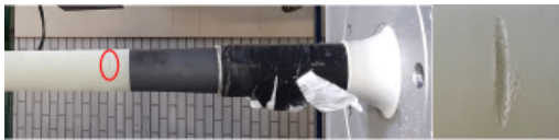
Continuous, Internal HV fault
