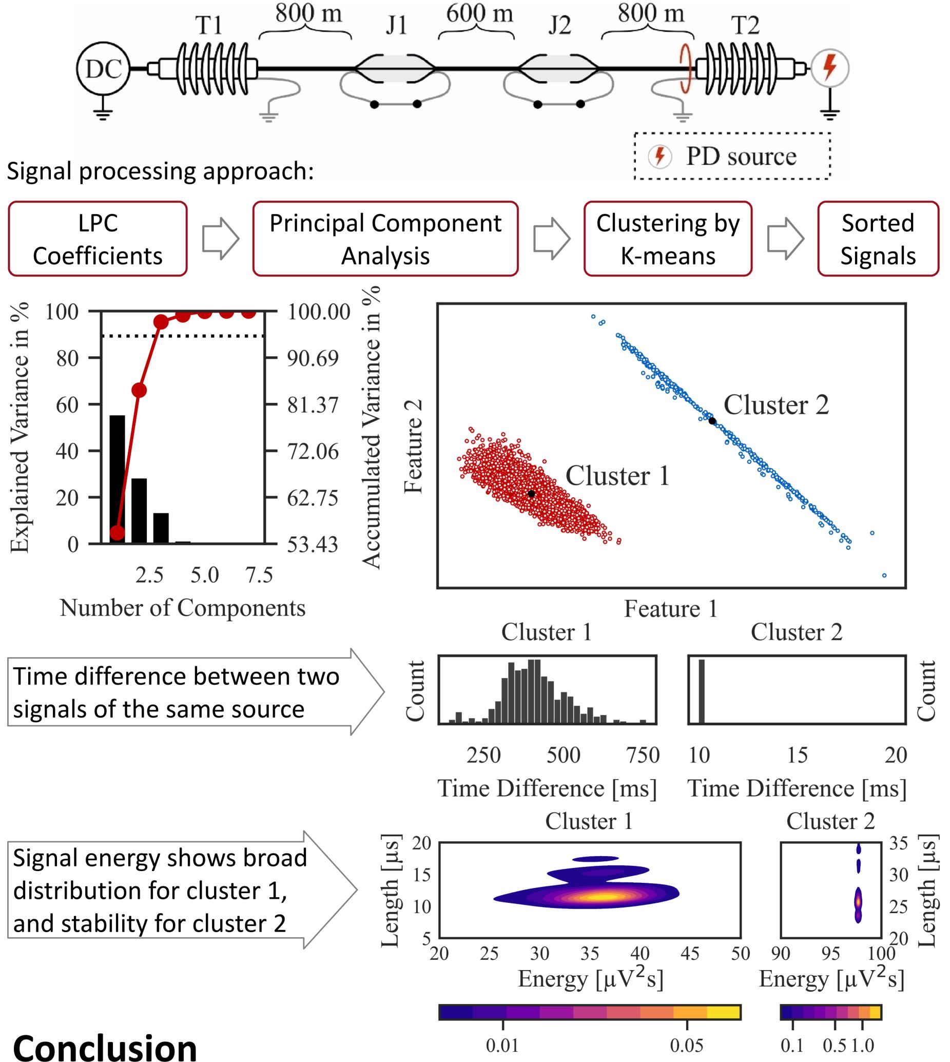
$\rightarrow$  Real-time signal processing and machine learning algorithms can be used to classify different PD sources and monitor their behaviour. This opens the road to predictive maintenance. http://www.cigre.org
