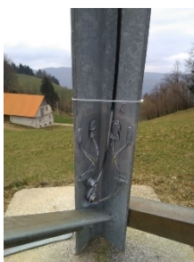
Fig. 4 Strain gauges at the location of the measured residual stresses on the L profile
