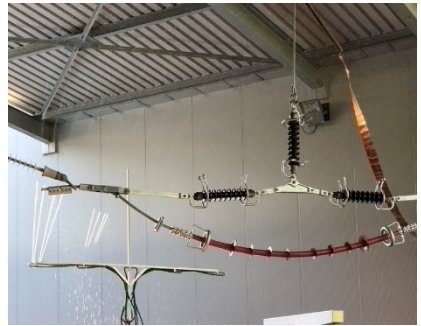
Wet AC type test at FKH-Laboratory in Switzerland
