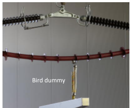
Bird test with a dummy at FKH-Laboratory in Switzerland
