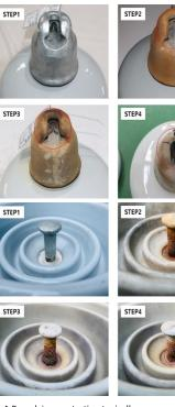
A Porcelain penetration typically appears on the inside edge of a cap where high electrical stress is present.
