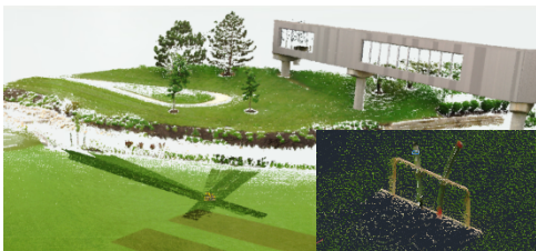
Figure 2 & 3: Manual registration of scan points ABCD (See Table 1) during open field testing and Bent pipe tool measuring diameter of conductor from scan points ABCD (See Table 1)
