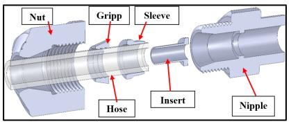
Printed kit and its nipple, exploded view
