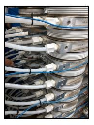
General view of the thyristors system with the refrigeration connections in detail
