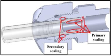
• Section view of the printed kit and its nipple (complete connector).
