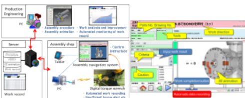
Figure 8 Digital work procedure for transformer
