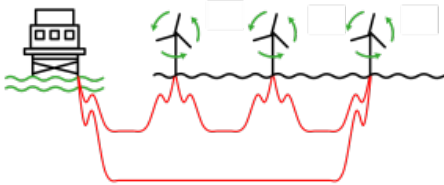
Loop Daisy Chain architecture
