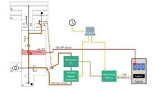
Injection of up to 1000 A single-phase test current to GIS bay via contacts of the isolated earthing switch
