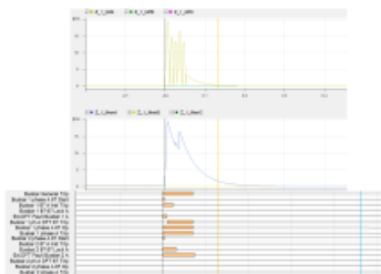
Figure 6. Busbar internal fault protection's response
