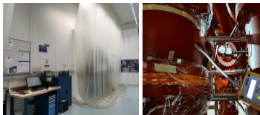
Accumulative method test (left hand side) and sniffing device test (right hand side).
