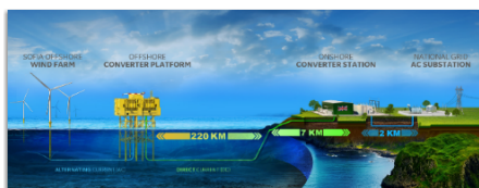
Figure-1 HVDC scheme link for Sofia
