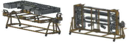
Special Tilting Device to move the new Valve Module through narrow corridor & entrance gate
