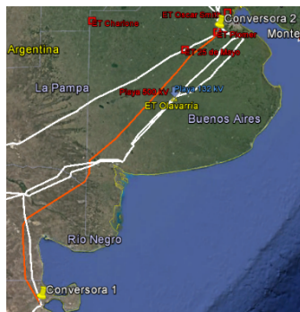
LCC technology of \pm 600 kV - 3000 MW - 1200 km
