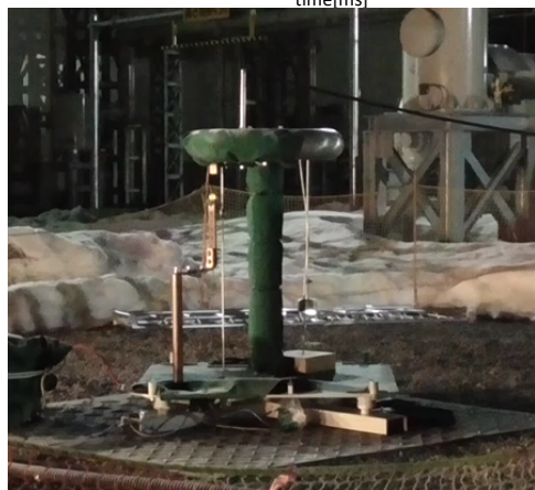
Ground fault generator during arcing
