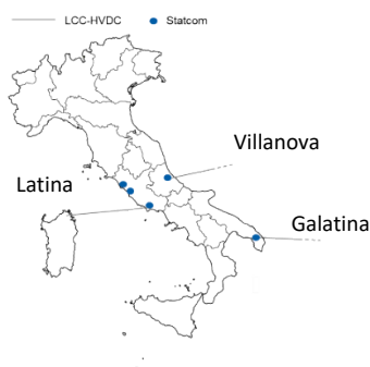
Figure 1—STATCOM installations planned and currently connected HVDC-LCC to the Italian network.
