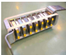
Figure 4-a : Group of 6 thyristors with bands, heatsinks and power connections
