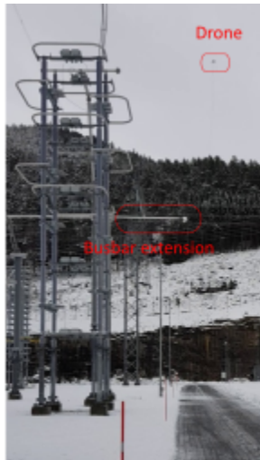
Field test arrangement for an overhead DC line fault at the negative pole 2 conductor at Ertsmyra converter station.
