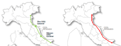
Left, DC conversion of a backbone situated nearby the Adriatic coast from South (Apulia) to North (Veneto) in synergy with the planned HVDC Adriatic Link; right reconstruction of a new 700 km OHL on the same route
