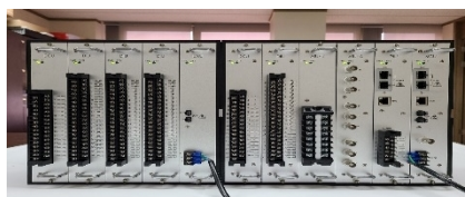
Figure 2. The MU for process bus of digital substation
