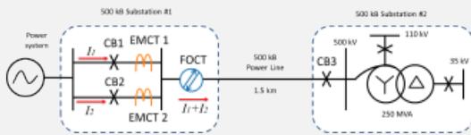
Fig. 7 Simplified single-line diagram describing a re-energization of a 250 MVA autotransformer
