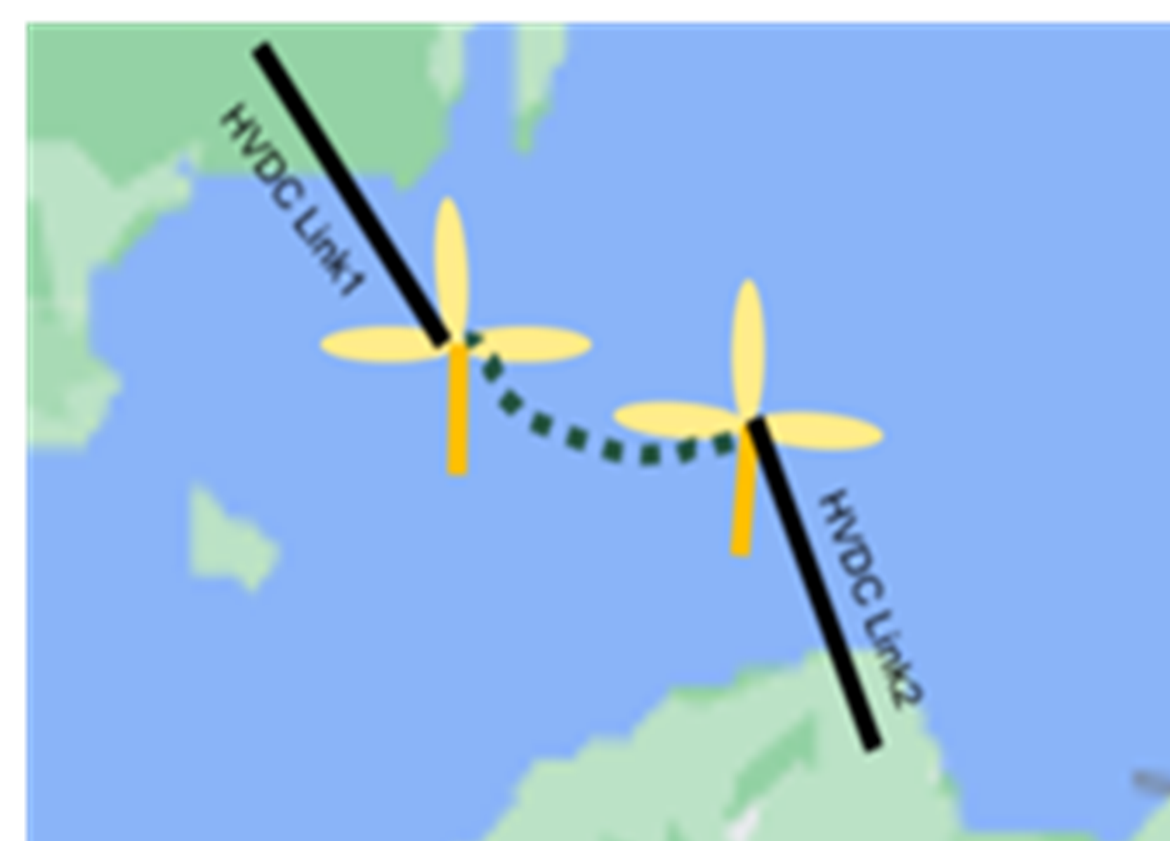
Figure 1-a. Interconnect two HVDC Links
