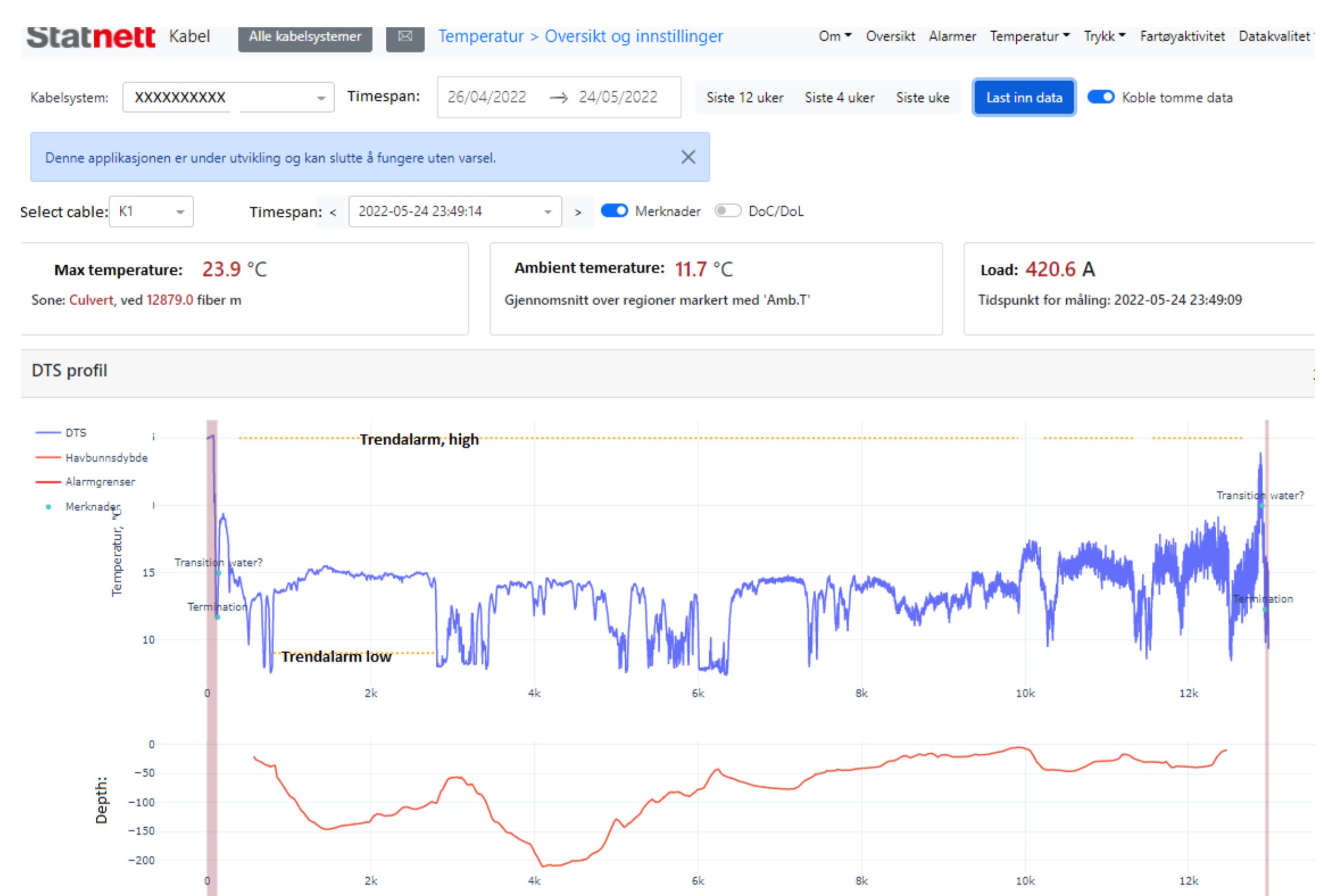
Figure 2: Overview of temperature profile for one selected subsea cable. Trend monitoring threshold alarms high/low added
