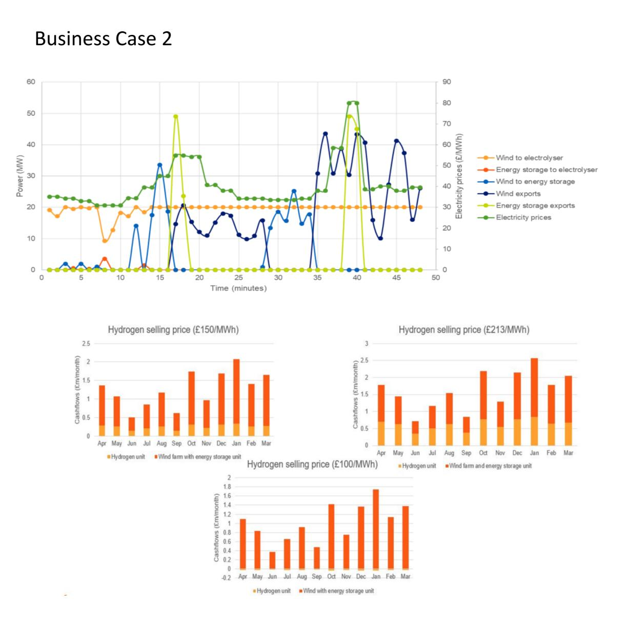
Overall, revenues of the joint unit depend on the size of the wind farm, electricity and hydrogen price magnitudes, electrolyser capacity and energy conversion efficiency of the energy storage unit. High hydrogen prices may encourage decision makers to prioritise wind to produce hydrogen and achieve higher overall profits.
