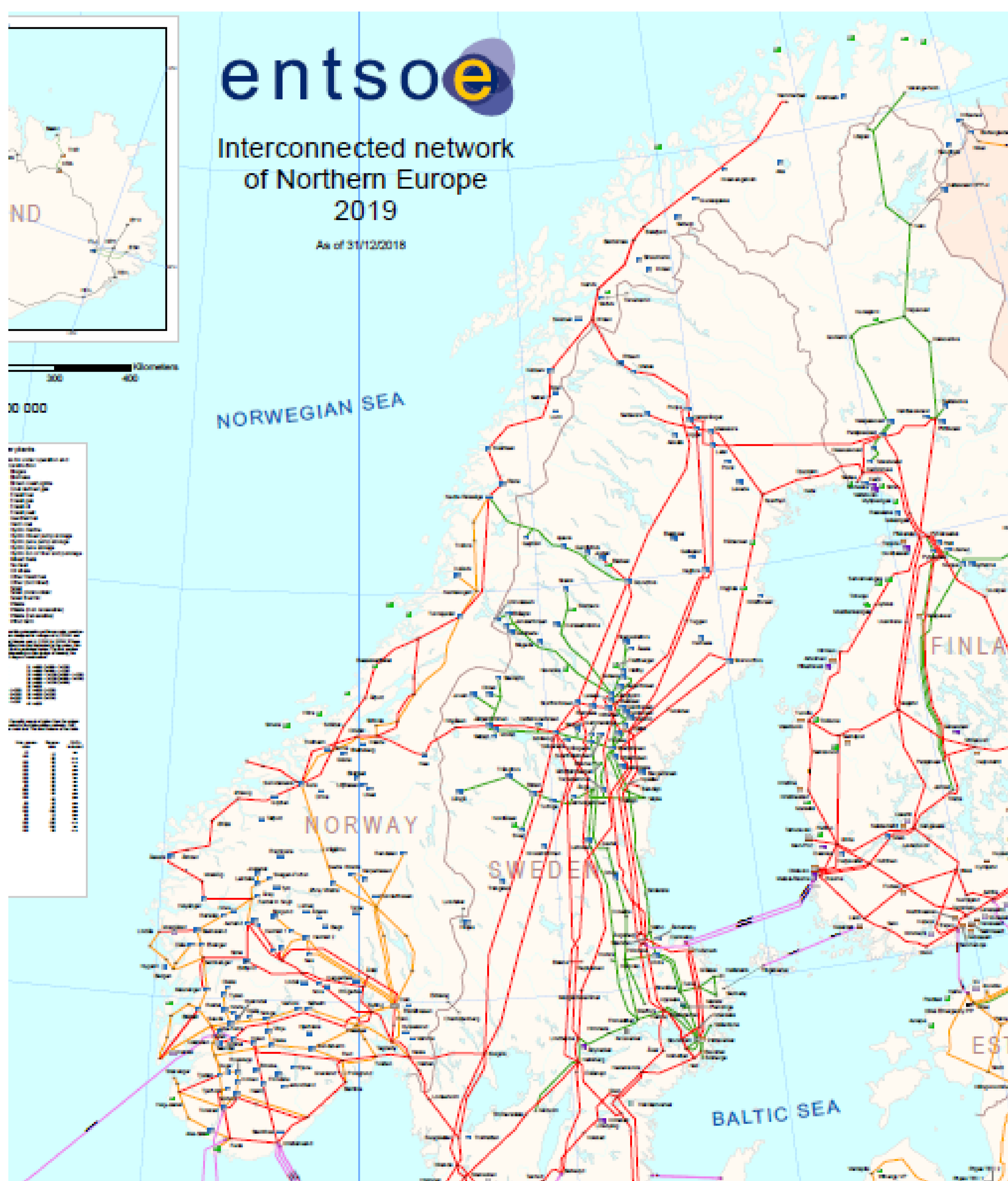
Norway transmission system with AC interconnectors to Sweden and HVDC connections to the European continent and UK
