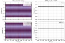
When performing HMIIF in a system with fundamental frequency components, care must be taken to remove this background component, so that only the relative impact of the harmonic injection is considered.
