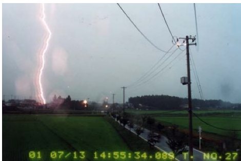
Direct lightning to distribution lines
