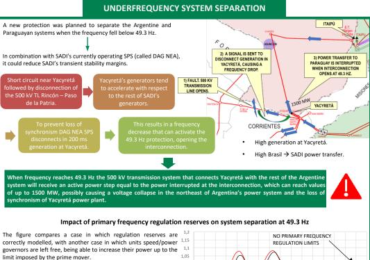
In the first case, the frequency will drop below 49.3 Hz, the 0.9 protection that separates the Argentine system from the 0.9 Paraguayan system will be activated **and the voltage collapse and** 0.85 loss of synchronism mentioned above could occur. In the second case, the units of the Argentine system would make an 0.75 extraordinary power contribution, the frequency will not reach 49.3 Hz and the system will evolve without losing stability.
