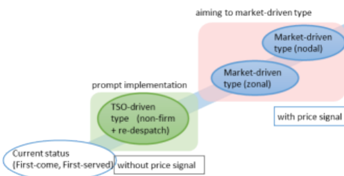
Figure 3 Congestion management considering Non-firm access
