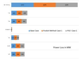
Comparing to the base case, reduction in control area wise net power loss was observed during both the cases in both pocket method and PSO.
