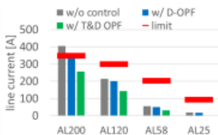
Figure 10. Line current in the provincial 2 distribution system
