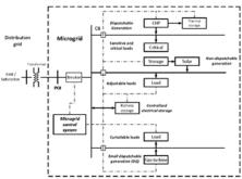
From (IEEE Std 2030.7, 2017). Group of interconnected loads and DER, with defined electrical boundaries, which acts as a single CONTROLLABLE entity with respect to the grid and can operate in interconnected or isolated mode
