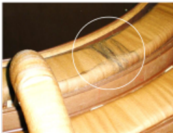
Figure 2 - Discharge mark caused by static electrification
