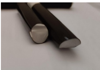
Fig 4. A broken test-bar ready for brakeage surface inspection.
