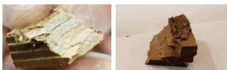
Examples of failed cellulose pressboard specimens exhibiting the slant shear type of failure
