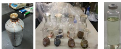
Figure 1. Ageing vessels: aluminium bottle (left), closed erlenmeyer flasks (middle), head space vials (right)
