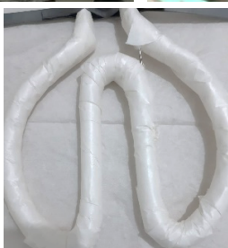
Test equipment developed for thermal fault modelling in liquid immersed insulation system: vessel with powerful water-cooling system + paper wrapped heating resistance
