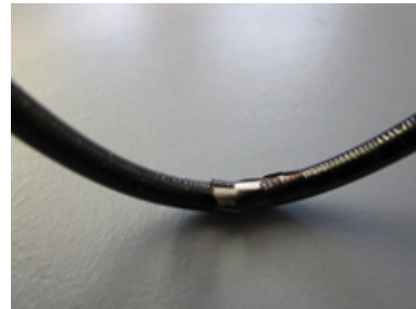
Cracking in a round enameled wire after a compatibility test.
