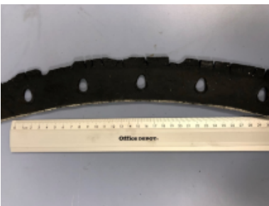
Material changes in an incompatible gasket, causing leakage.
