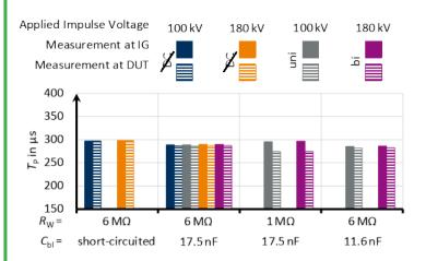
• Without applied DC voltage: Shorter peak times at the IG and larger at the DUT with increasing ignition voltage of the spherical spark gap
