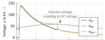
• Differences in the time parameters between uni- and bipolar superposition because of the different ignition behaviour of the spherical spark gap
