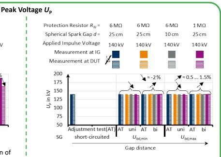
Deviations of U<sub>p</sub> between IG and DUT are significantly smaller when using a SG instead of a blocking capacitor
