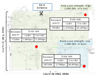
Fig. 7 Measurement of private LTE radio propagation characteristics in a thermal power plant
