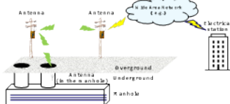
Fig. 1 Application image of wireless communication at a manhole for underground power transmission line facilities.
