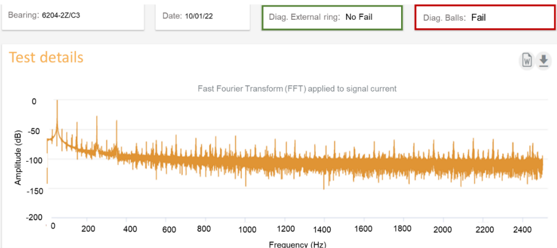
Figure 10. Diagnosis result for a IM with dirty bearing
