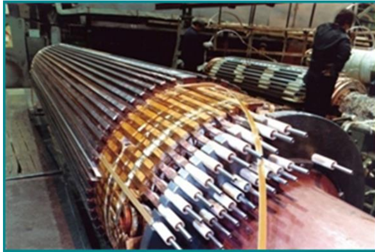
Fig. 5. General View of the Rotor Winding of the T3B Turbine Generator
