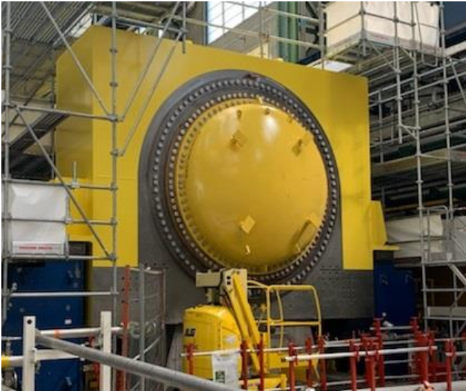
Fig.10. Test of stator during assembly on the test bench for running test
