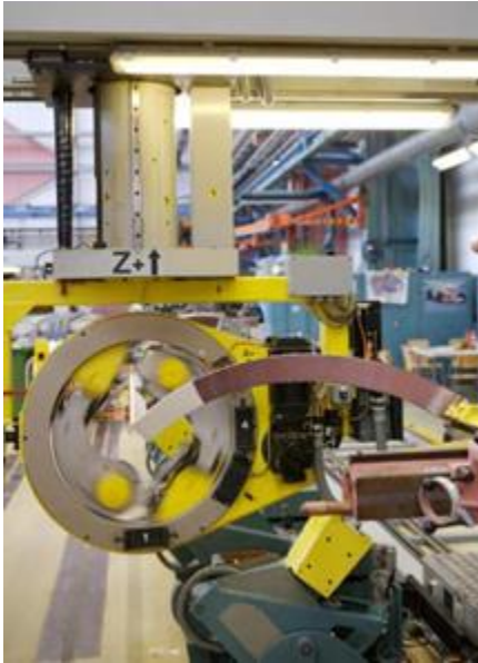
Fig.3. Stator bars insulation manufacturing process
