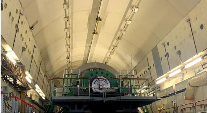
Fig.9 Test of rotor at balancing pit
