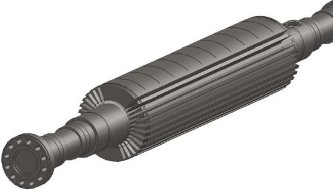
Figure 11. Rotor forging – general view
