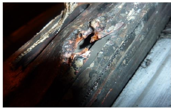
Figure 5. Molten copper from slot 11
