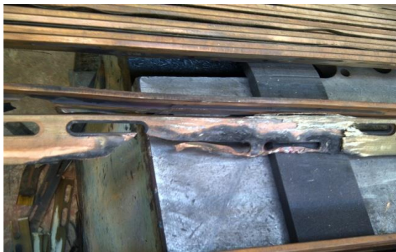
Figure 4. Molten copper from slot 24
