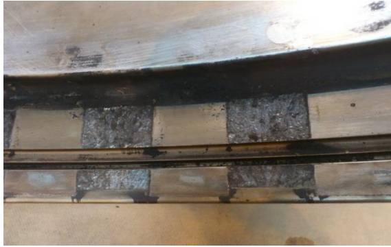
Figure 2. Molten retaining ring fit area
