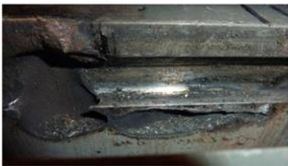
Figure 6. Molten tooth in slot 11
