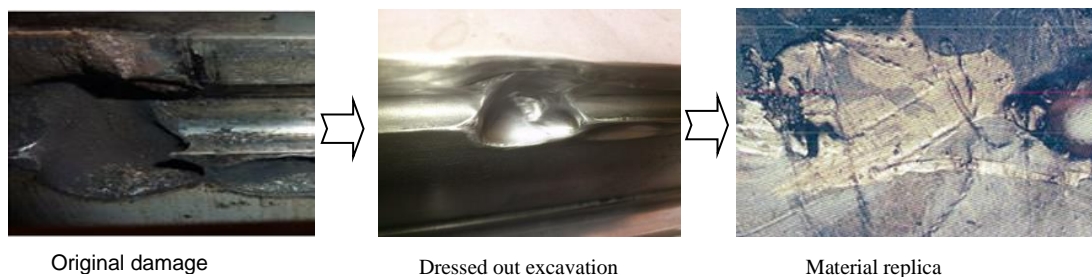
Figure 8. Earth fault location recovery process
