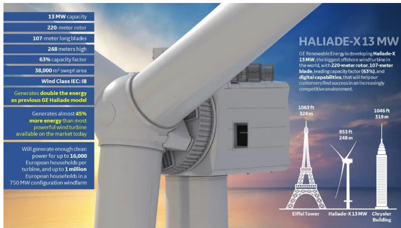
Figure 1- Comparative size of the Haliade-X wind turbine [1]
