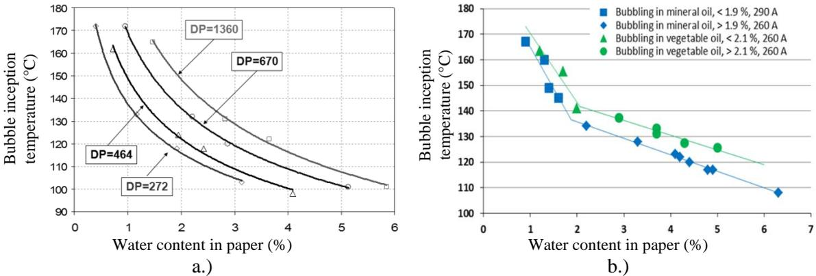
Figure 1: a.) Impact of the degree of polymerisation (DP) and b.) alternative insulating liquids on the bubble formation temperature, adapted from [6, 7].
