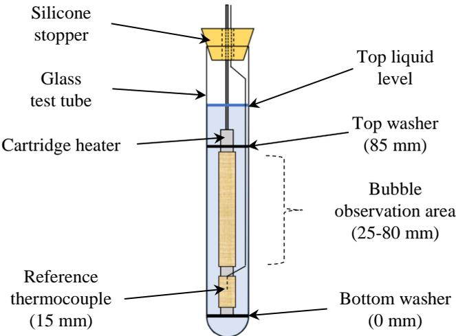
Figure 2: Test setup sketch.
