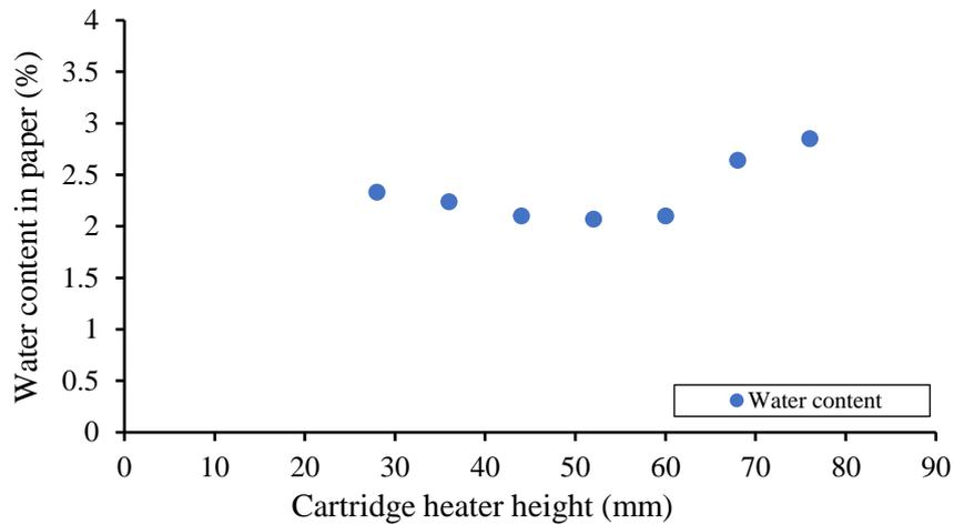
Figure 8: Water content in paper of the observation area after being heated.
