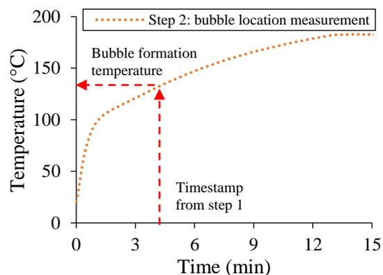
Figure 6: Correlation of measurement step one and step two to obtain the temperature at the bubble formation location.
