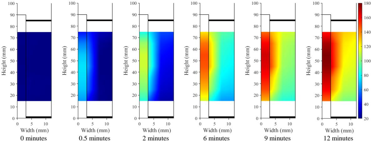
Figure 4: Several heat maps generated from the measurements show the temperature development within the sample during a heating cycle.
