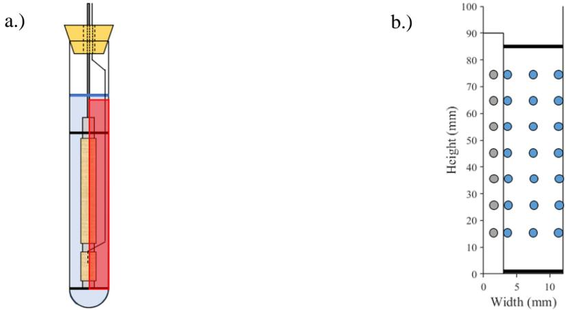
Figure 3: a.) Sketch of the test setup with highlighted area for the illustration b.) of the individual locations from the thermocouples.
