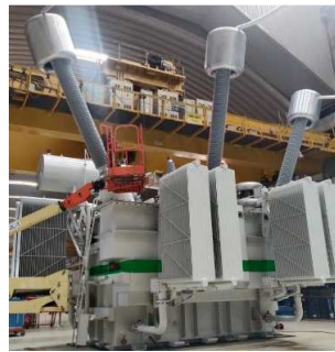
Figure 9: Fully assembled 50MVA reactor under testing.
